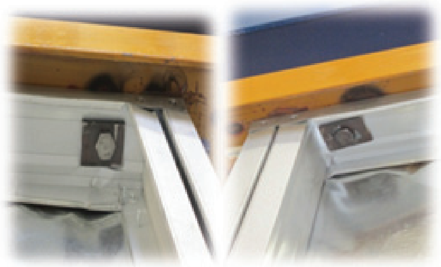
Figure 9. Failure modes of specimens type II a. Top and bottom local buckling; b. tearing of the bottom track's flange b
