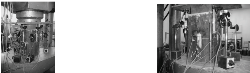
Fig. 2. Test stand: a) circular hollow cross-section members, b) square hollow cross-section members
