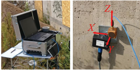
Fig. 5. Data acquisition system LMS SCADAS (left) and accelerometer PCB model 356B18 (right)
