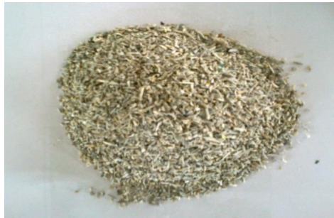
Fig.1.Polymer Industries Waste (PIW)
