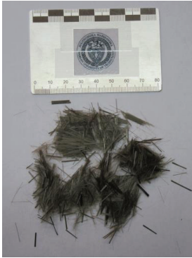
Fig. 1. Basalt-polymer fibers with a length of 12 mm
