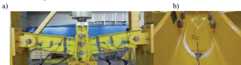
Fig.24. P-5 specimen: a) view before ending test, b) column view after test
