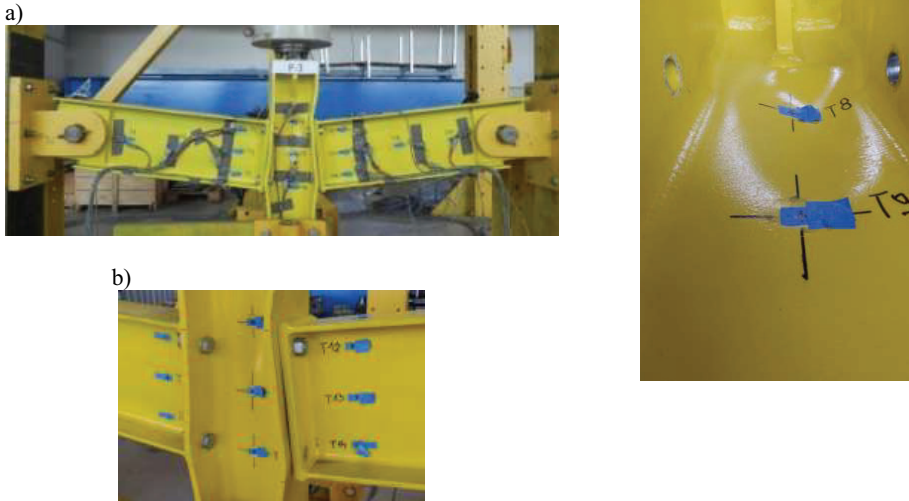
Fig.15. P-3 specimen: a) view before failure, b) failure mode of specimen, c) column view after test
