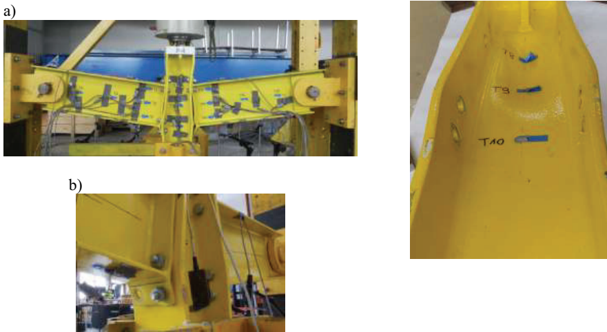
Fig.18. P-4 specimen: a) view after failure, b) failure mode of specimen, c) column view after test
