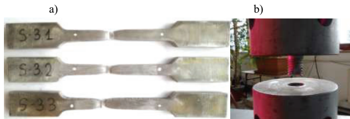
Fig. 7. View: a) material coupon after test, b) bolt after test
