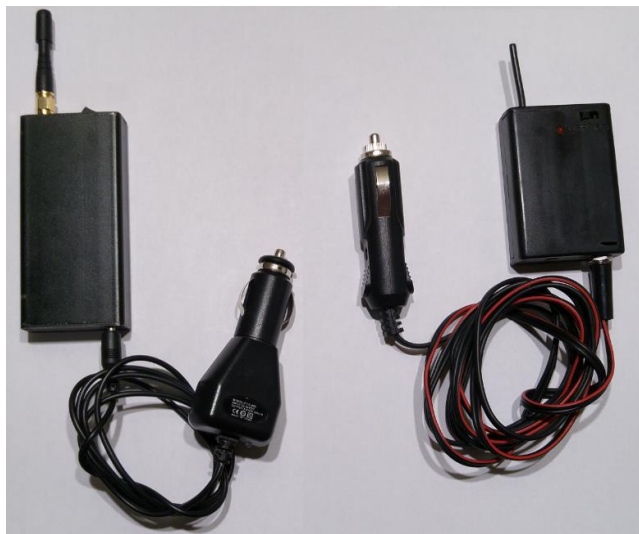
Fig. 15. GX-40B by TTS jamming device and Spy Electronics LTD jamming device
