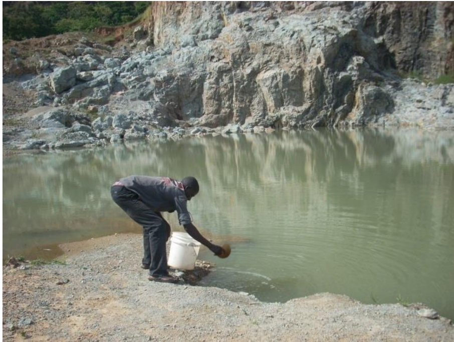
Plate I: Water pond from a quarried section of a rhyolite. This rock is the major contributor of fluoride in drinking water in Langtang area
