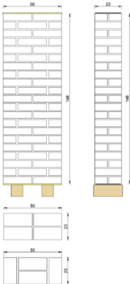
Figure 6. Dimensions of the finished masonry specimens.
