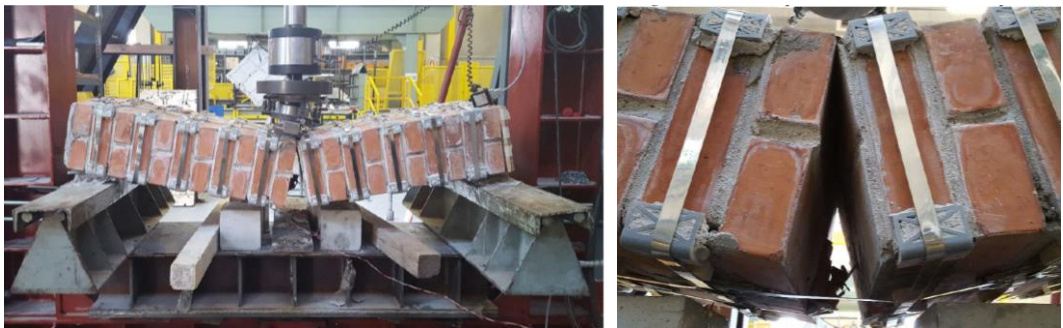
Figure 11. Deformation of the specimen P1 during bending test: zoom of the central part on the right.
