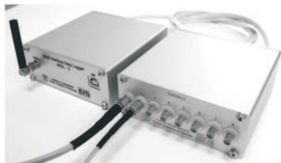
Fig. 7. Constituents of a telemetric soil moisture, salinity and temperature monitoring station: an eight-channel TDR meter of the TDR/MUX/mpts type together with a GPRS modem MIDL-2 type.
