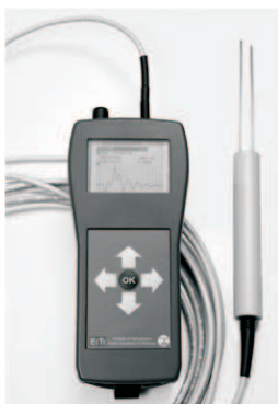
Fig. 8. Handheld TDR meter for soil moisture, salinity and temperature type FOM/mts together with a measurement probe type FP/mts.
