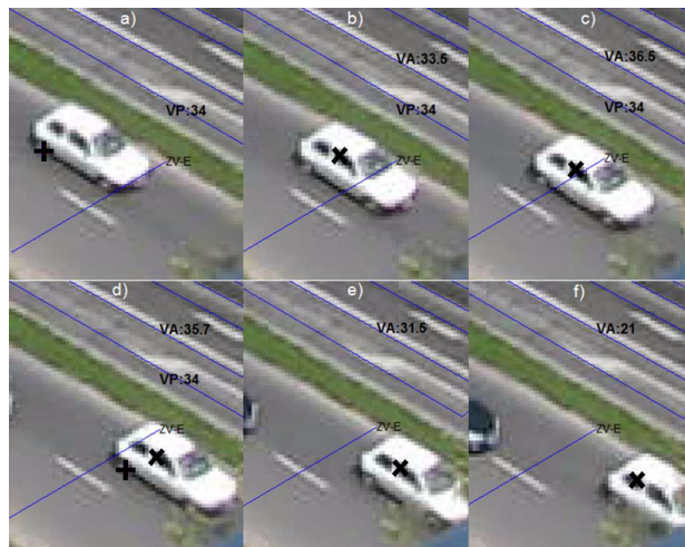
Fig. 6: Comparing the data needed for velocity calculation: x - tracking the center of gravity by the video detector, + - characteristic point localizations obtained from GTGT
