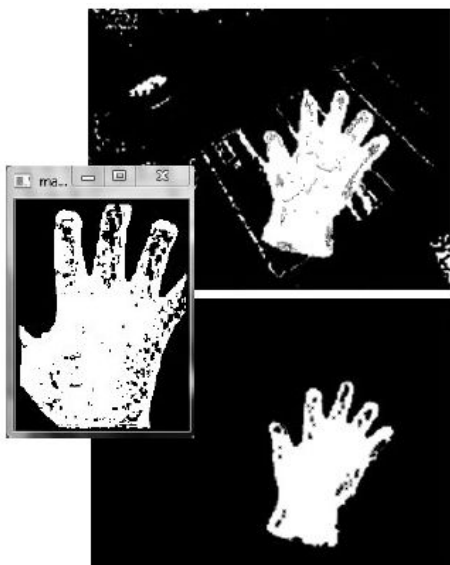
Fig. 7: The image after back projection (at the top) and its copy which was processed with a mask created based on threshold operation (at the bottom)
