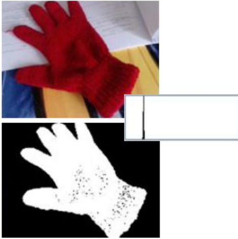
Fig. 3: The result of the back projection based on the histogram which was created for the searched object. In this case it was a red glove
