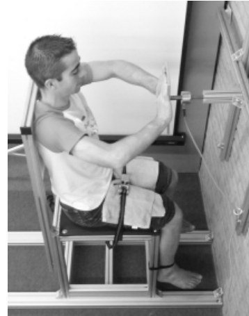
Fig. 1. Generic test to measure the strength of the upper limbs extension with (portrayed) and without backrest support
