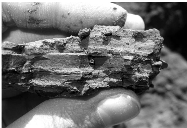
FIGURE 1. Varved clay and its laminated structure
