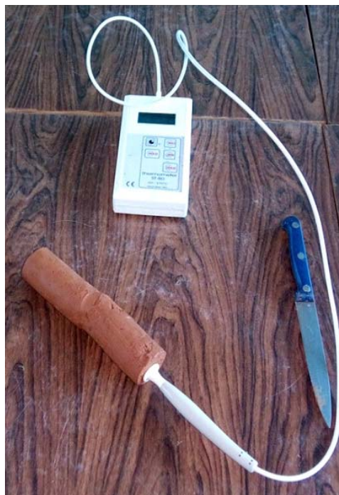
FIGURE 1. The test-bench for measuring changes in the temperature of the frozen soil
